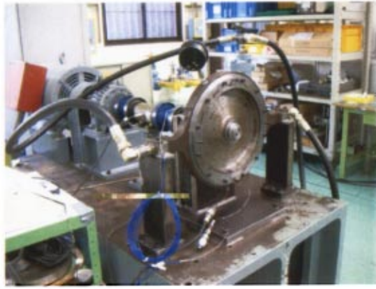
Fig. 12 Seal rotation test device
