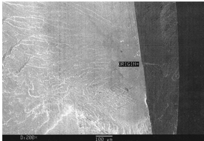
Fig. 4 SEM photo showing ridge HCF initiation
